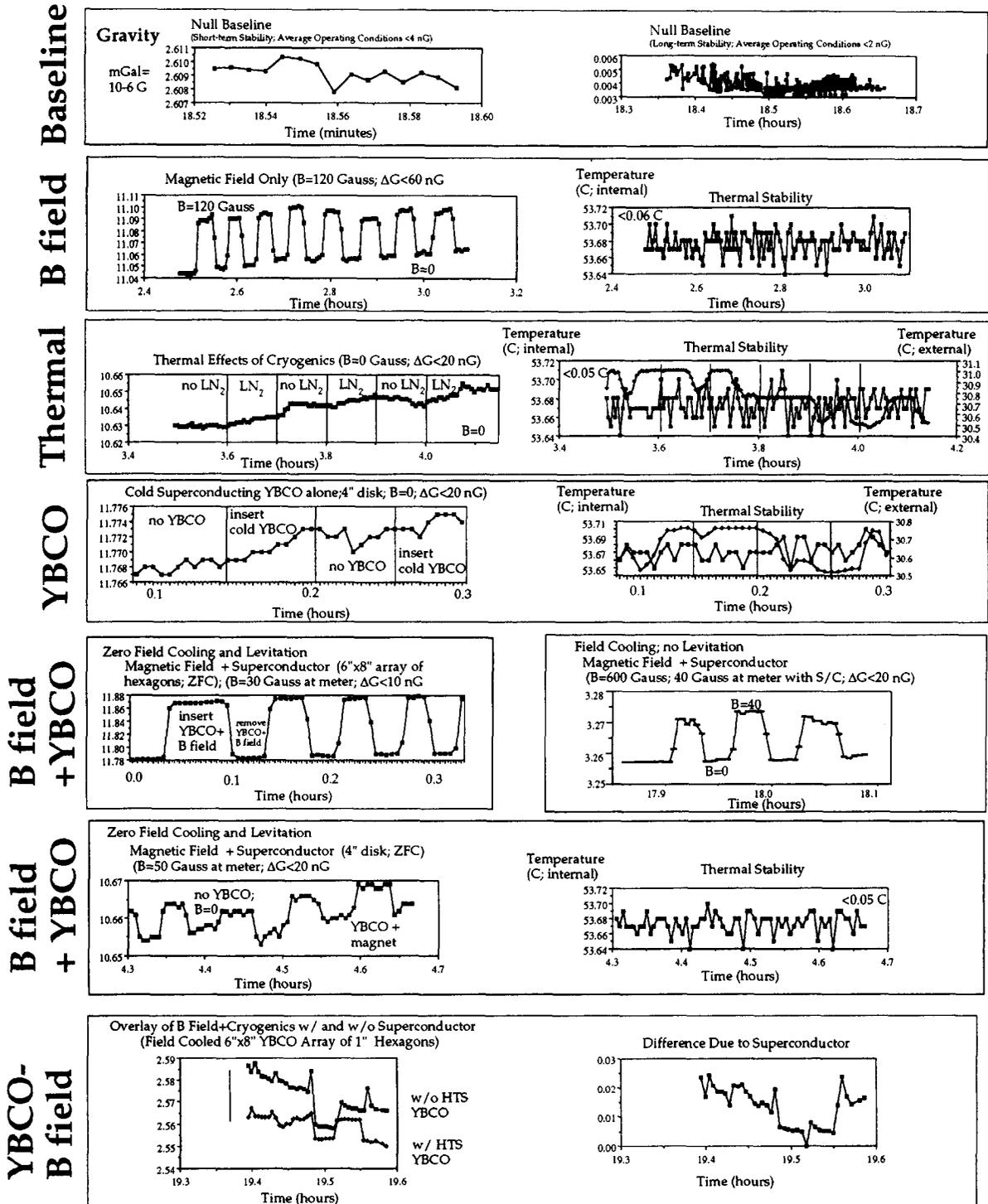
Fig. 3. Experimental results for measured DC magnetic field and gravimeter fluctuations (baseline plus magnetic, thermal and superconductive contributions). If not otherwise indicated the vertical axis is apparent gravity in units of mGals or  $10^{-3} \text{ cm s}^{-2}$ . See text for protocol details.
