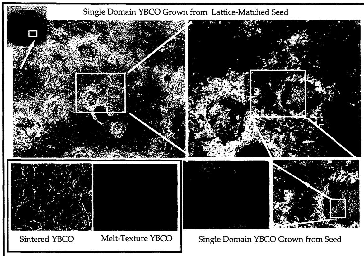
Fig. 1. Scanning electron microscopy of hexagonal, single-domain YBCO superconductor at increasing magnification. Surface machining textures the domain.
