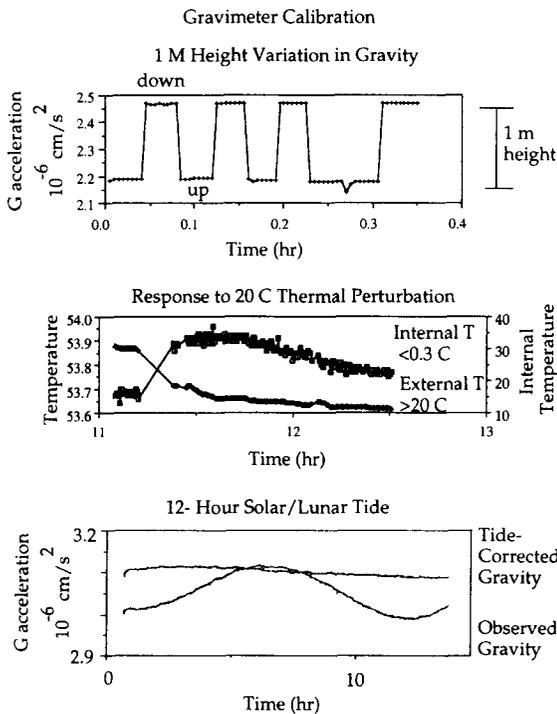
Fig. 2. Calibration and proof-testing gravimeter: (1) altitude variation of 1 m and resulting gravity change ( $3.08 \times 10^{-7} \text{ cm/s}^2$  per m altitude); (2) thermal constancy of gravimeter interior during  $20^\circ\text{C}$  external temperature change; (3) solar and lunar tide during long duration reading (12 h).
