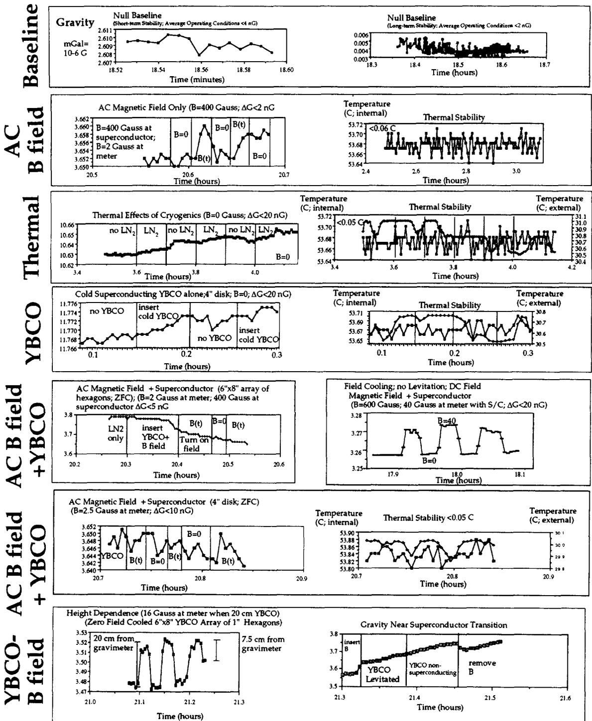
Fig. 4. Experimental results for measured AC magnetic field and gravimeter fluctuations (baseline plus magnetic, thermal and superconductive contributions). If not otherwise indicated the vertical axis is apparent gravity in-units of mGals or  $10^{-3} \text{ cm s}^{-2}$ . See text for protocol details.
