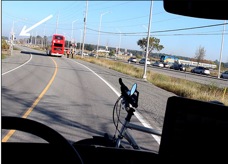
Photo 12. Traffic sign obscuring back lights
