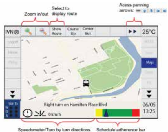
Photo 20. Transit control head display
