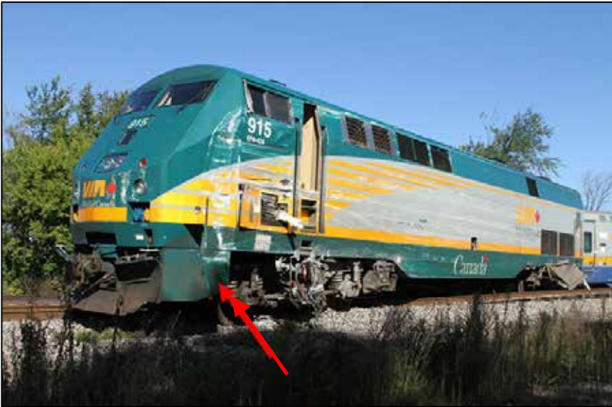
Photo 5. Damage on locomotive VIA 915
